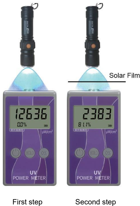
Figure 1. Measure the UV rejection performance of window film
