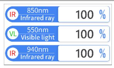
Select "550nm/850nm", the measurement interface display 550nm visible light transmittance, the 850nm infrared transmission;
