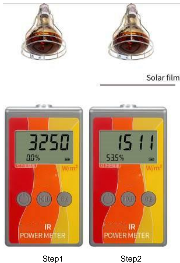
Figure1: Measuring the infrared rejection rate of solar film
