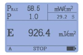
In the STOP interface, long press the "POWER" button to power off the meter.
