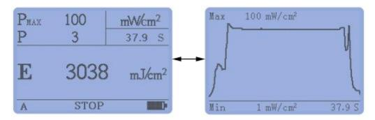
In the stop status, long press the "ENTER" key to clear the current test data.
