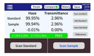
In the measurement interface, press the "Scan Standard" button to set current value as standard. Press the "Scan Sample" button to use current value as sample. If short press the button on the right side, another measurement will also be taken and the current value will replace the previous one. When measuring or adding a standard and measuring a sample, the difference or color difference between the two measured values will be calculated with the following results:
