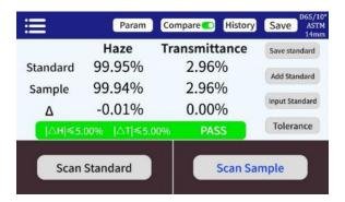
In the measurement interface, press the "Scan Standard" button to set current value as standard. Press the "Scan Sample" button to use current value as sample. If short press the button on the right side, another measurement will also be taken and the current value will replace the previous one. When measuring or adding a standard and measuring a sample, the difference or color difference between the two measured values will be calculated with the following results:
