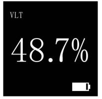
**VLT/UVT/IRT:** The measurement interface displays VLT (visible light transmittance), UVT (ultraviolet transmittance), 940IRT (940nm infrared transmittance), 1400IRT (1400nm infrared transmittance).
