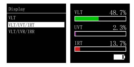
**VLT/UVR/IRR:** The measurement interface displays VLT (visible light transmittance), UVR (ultraviolet rejection rate), and IRR (infrared rejection rate).
