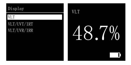
**VLT/UVT/IRT:** The measurement interface displays VLT (visible light transmittance), UVT (ultraviolet transmittance), and IRT (infrared transmittance).
