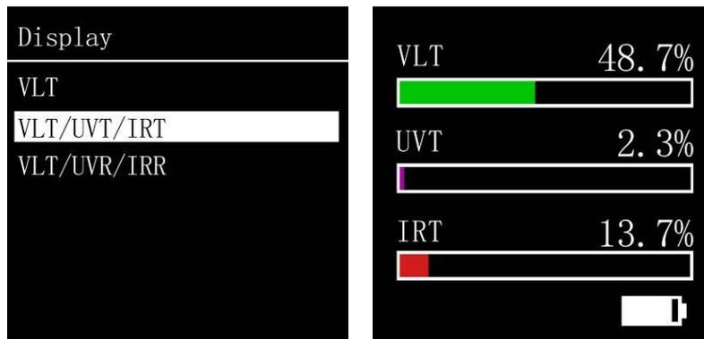
**VLT/UVR/IRR:** The measurement interface displays VLT (visible light transmittance), UVR (ultraviolet rejection rate), and IRR (infrared rejection rate).
