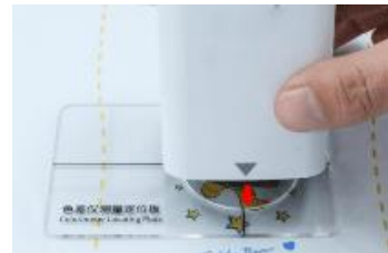
Place the meter on the positioning hole
