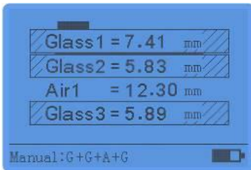
Laminated glass with one layer air
