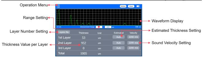
Thickness measurement results of 3 layers
