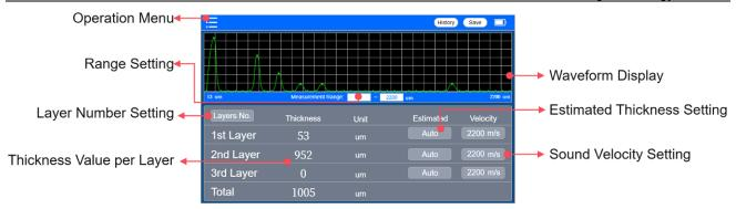
Thickness measurement results of 3 layers
