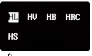
**Calibration**: Short press the  $\underbrace{\textcircled{b}}_{\text{Enter}}$  button to enter the calibration interface, the screen prompts [Please measure the standard hardness block] and flashes, then you can measure the standard hardness block (single or multiple times). After measurement, the cursor moves to the actual value area, then
