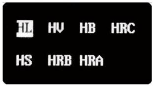
Calibration: Short press the Enter button to enter the calibration interface, the screen prompts [Please measure the standard hardness block] and flashes, then you can measure the standard hardness block (single or multiple times). After measurement, the cursor moves to the actual value area, then press Enter or ▼ button to adjust the actual value to the standard value of the hardness block. Long
