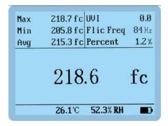
• In the measurement mode, if the backlight is off, press the button to light the backlight; if the backlight is already lit, short press the button, the interface switches to the spectral curve interface, which displays the spectral curve, correlated color temperature (CCT), color rendering index (CRI), standard deviation of color matching (SDCM), and blue light hazard ratio.
