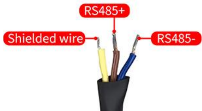
(Description of Communication Cable Cores)
